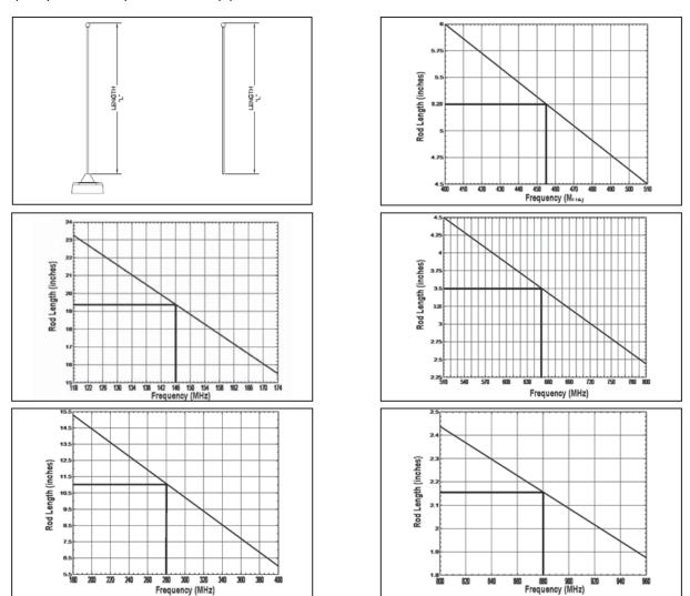
The dark line indicates the approximate length for the rod (y-axis) to the tuned frequency (x-axis)
