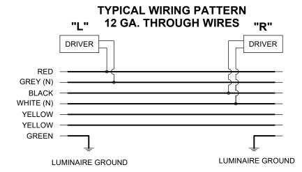
YELLOW WIRES FOR 3-WAY SWITCHING INCLUDED ON "2Y" FIXTURES ONLY
